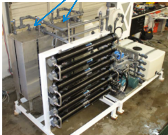
5000-10,000 gpd PFO pilot system (20-40 m 3 /day) (with two 42 m 2 modules)
